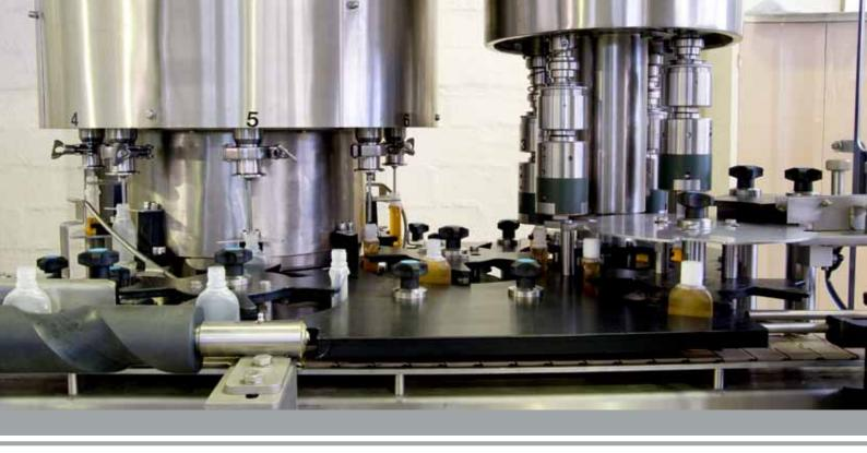
Level Filler option: Level filling turrets are used for low viscosity liquids only. The containers are lifted on a cam, thus opening the level nozzles with filling automatically stopping at the required fill height. The fill height is simply adjusted by adding or removing spacer rings from the nozzles.
