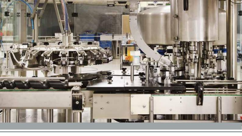
The *RFC Series* of monobloc rotary rinsing, filling and capping machines is the result of over 15 years of activity in the field of liquid filling. The RFC Series is supplied in two versions: The RFC-P series is for pharmaceutical applications and the RFC-G Series is for food, beverage, cosmetic, personal care and home care applications.
